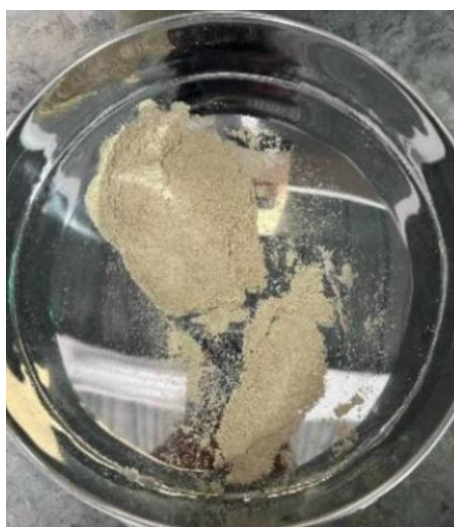
Figure 1. Treated corn husk powder (alkali and silane treated) ready for mixing with acrylic powder
