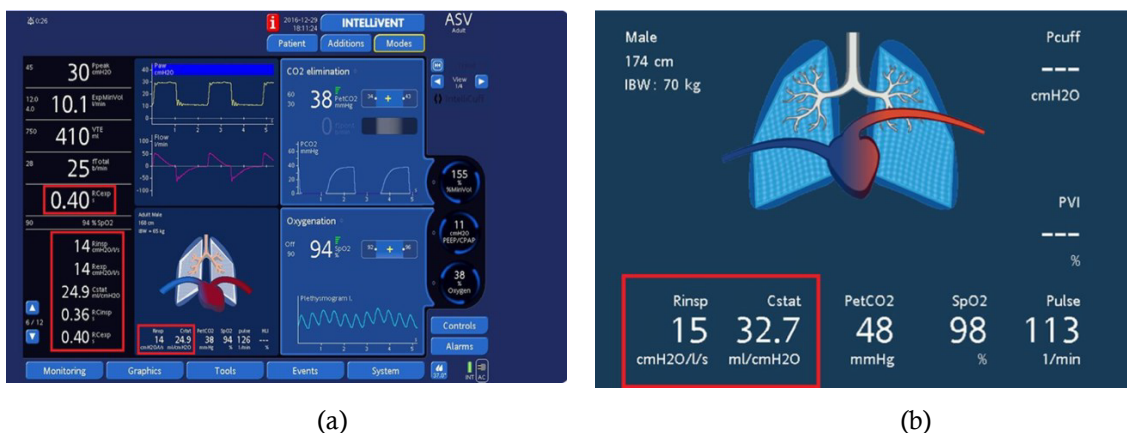
Figure 10. (a) Dynamic Lungs Monitoring Panel on a Mechanical Ventilator showing (b) trends for all respiratory mechanics variables (Arnal et al. , 2018).
