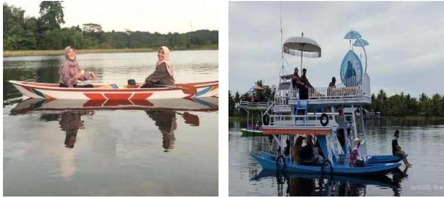
Figure 2. Difference between Original Gubang and Two Hull Gubang Source: Personal Documentation and Gubang Park Management
