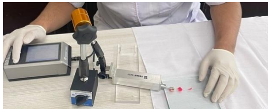
Figure 2. The sample measurement process was performed using a surface roughness tester.
