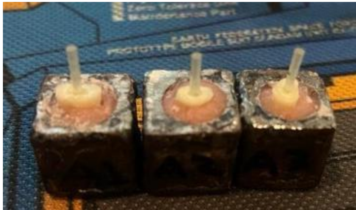
Figure 1. Samples were mounted in the acrylic block prior to the pull out test
