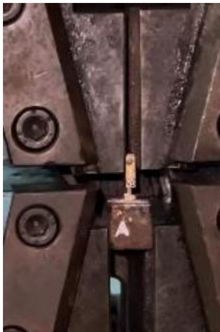
Figure 2. Pull out test using Univeresal Testing Machine (TN20 MD)
