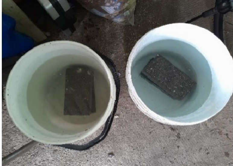
Figure 1. The sample being tested for absorption capacity.
