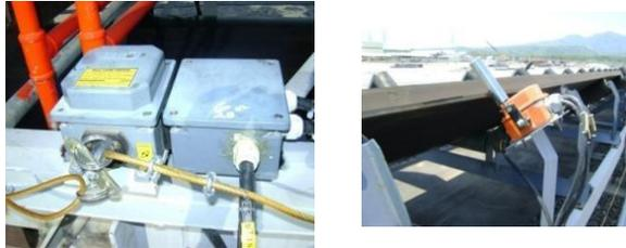
Gambar.1. *Pullcord Switch* dan *Belt Sway Switch*
