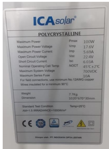
Gambar 5. Spesifikasi solar panel ICA Solar 100 Wp
