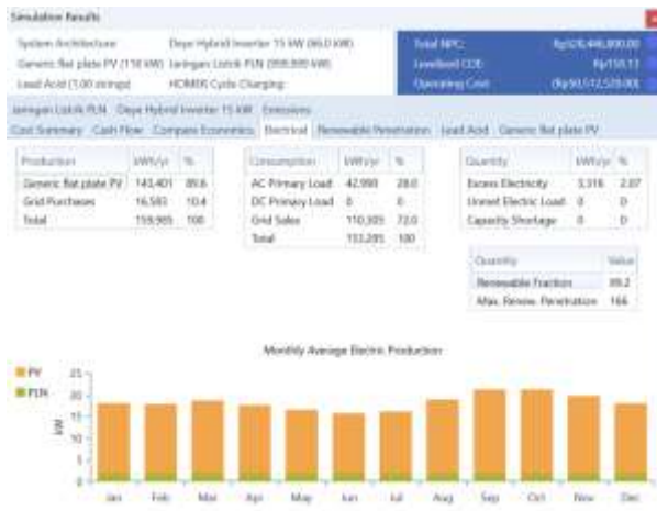
Figure 7. Electrical Production of Configuration 2
