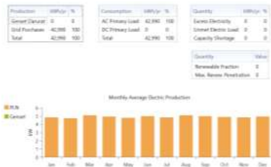
Figure 8. Electricity Production Combination of PLN Electricity Network System and Emergency Generator
