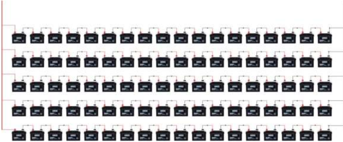
Figure 3. Battery System Circuit
