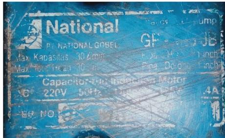
Gambar 6 Nameplate Pompa Air merek National daya listrik 125 watt
