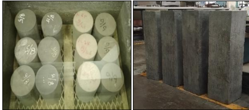
Fig. 2. Curing of test specimens: compressive strength test specimens and composite columns specimen.
