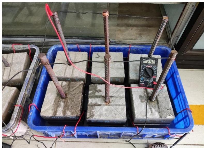
Fig 10. Accelerated corossion test (ACT)
