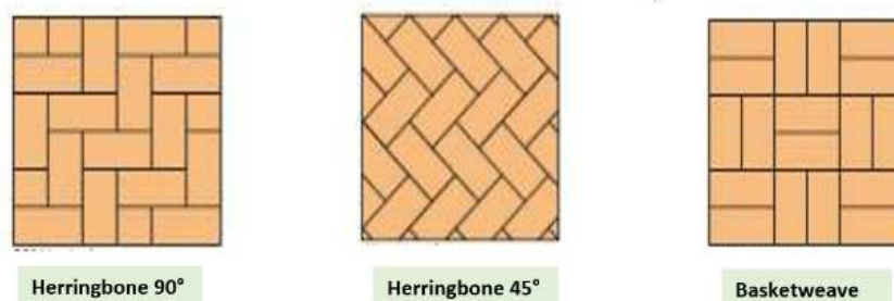
Fig. 6. Horizontal and Vertical Pavement Pattern Model Installation
