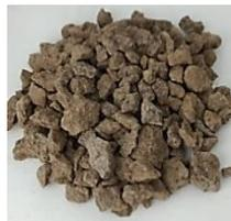
**Fig. 3.** Artificial Coarse Agreggate (ACA)
