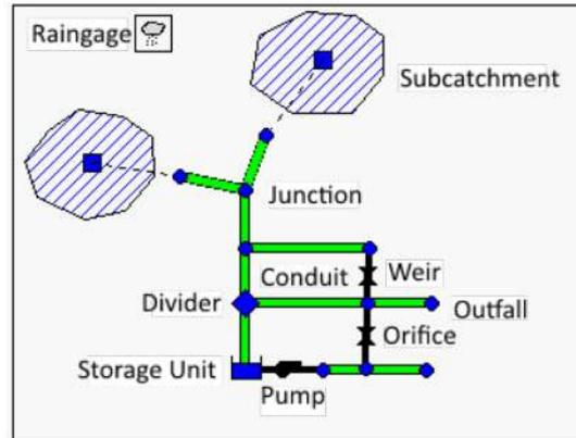
**Fig. 1.** SWMM's conceptual model of a stormwater drainage system.
