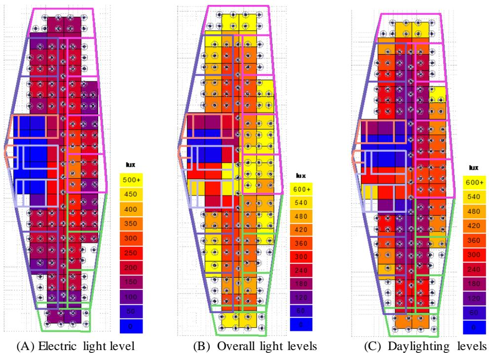
Figure 4. Lighting Analysis on typical floor (Model 1)
