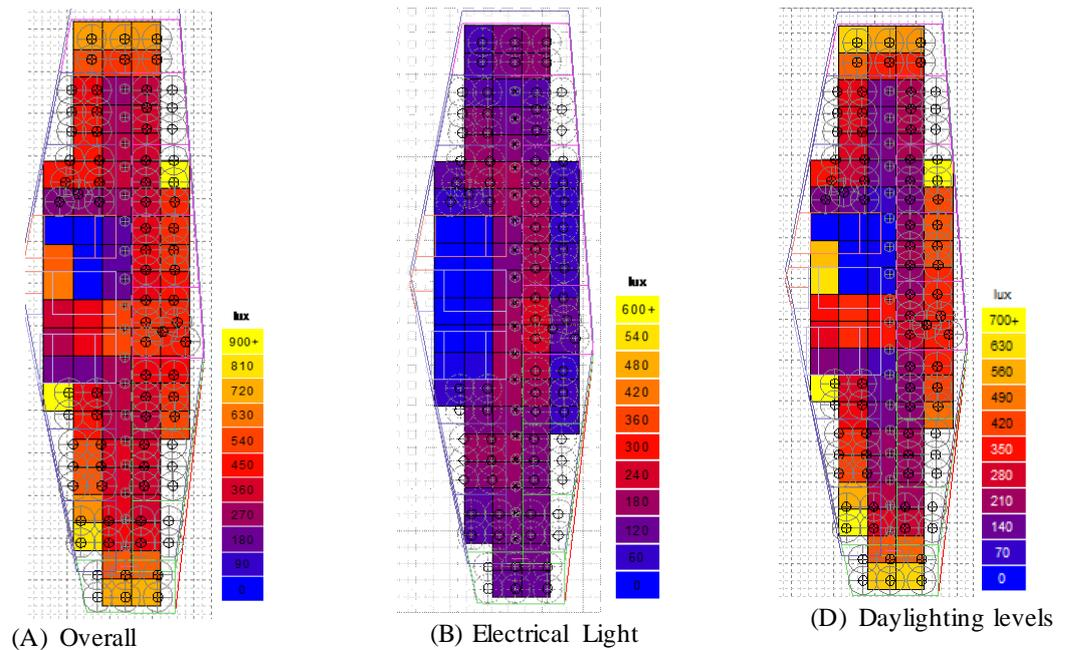
Figure 6. Lighting analysis on typical floor (Model 2)
