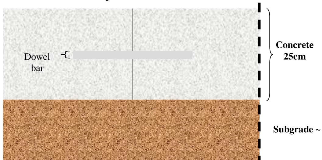
Figure 7. Rigid pavement structure layer thicknesses over stabilized subgrade
