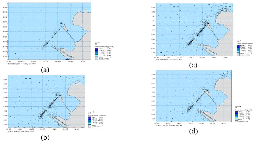
**Fig. 5.** The pattern of sediment transport in (a) flood toward ebb (b) lowest ebb (c) ebb toward flood (d) highest flood (Source : Data Processing, 2016)
