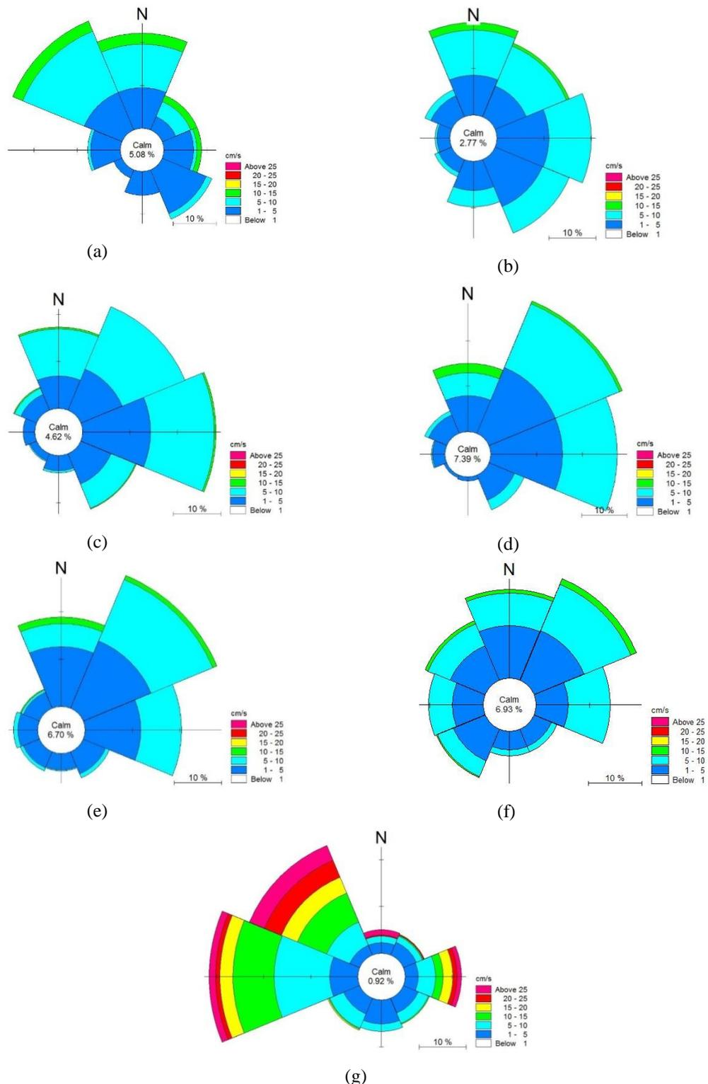
**Fig. 2.** Currentrose of depth a) Cell 1 (7,0 – 8,0 meter); b) Cell 2 (6,0 – 7,0 meter); c) Cell 3 (5,0 – 6,0 meter); d) Cell 4 (4,0 – 5,0 meter); e) Cell 5 (3,0 – 4,0 meter); f) Cell 6 (2,0 – 3,0 meter) g) cell 7 (1,0 – 2,0 meter) Tanggal 3 Juni 2016 – 6 Juni 2016 (Source : Data Processing, 2016)
