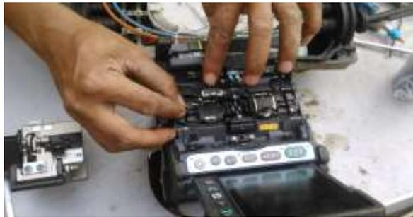
Gambar 11. *Fusion Splicing*
