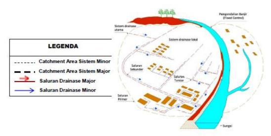
Figure 1. General Lay-out of Urban Drainage System
