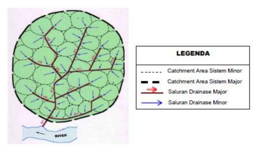
Figure 2. Schematic lay-out from minor and mayor in urban drainage system
