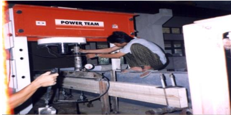
Picture 1: The Image of Glulam Beam Test.
